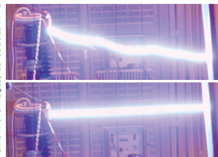
Image of a high-voltage electrical discharge, that is, artificial lightning, over a distance of 3 m with (straight path) and without (erratic path) the assistance of a guiding laser filament.
