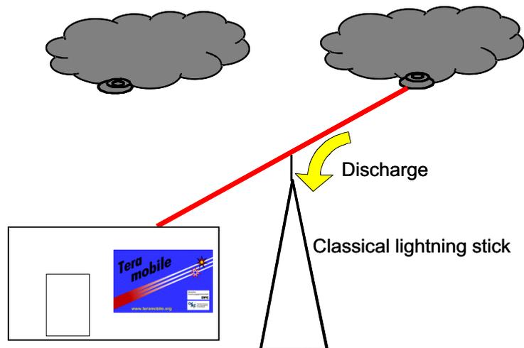
Figure 12: Possible setup of a field experiment to try the control of real atmospheric lightning.
