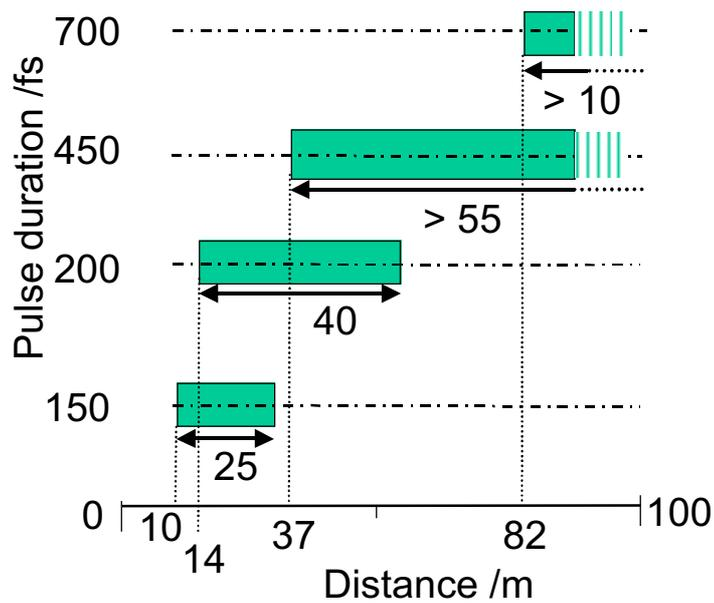
Figure 3: Chirp dependence of the filament position and length. The shortest pulse in the experiment was approx. 100 fs long. Here the value 150 fs stands for a slight positive chirp, the three upper durations represent the length of pulses with negative chirp.
