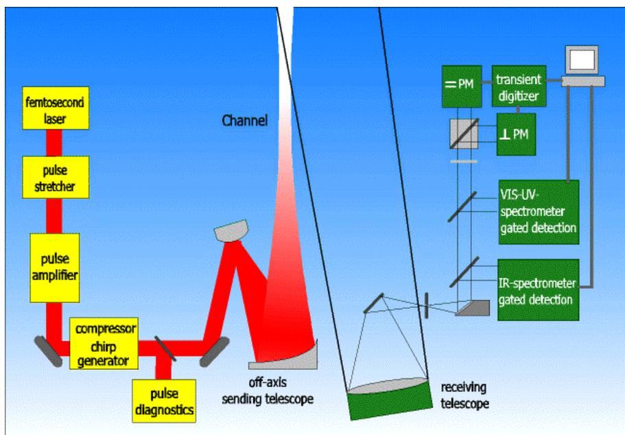
Figure 1: Schematic diagram of the femtosecond lidar setup.
