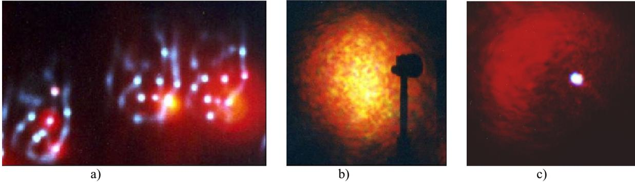
Figure 2: Beam profiles of TW pulses propagating through air (real color photographs taken from a white screen).
