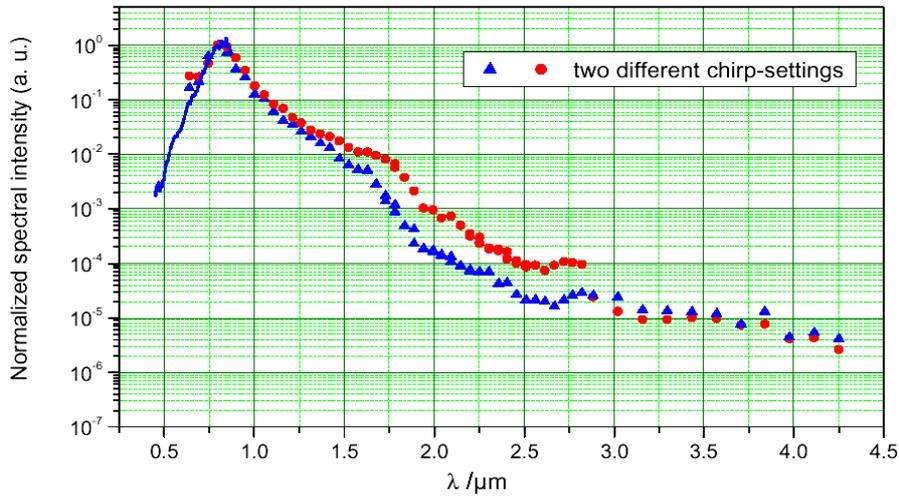
Figure 4: Measured spectra of 2-TW pulses after propagation of 30 m behind a 10-m lens. The triangles represent unchirped pulses, the circles pulses with a negative chirp (both after compressor; the negative chirp mainly compensates the dispersion in the lens).
