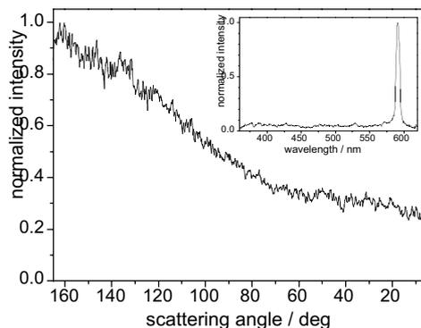
Figure 9: Angular distribution of 589-nm light from a microdroplet containing a 5 molar NaCl solution. The droplet was excited by a focussed laser beam ( $4 \cdot 10^{14} \text{ W/cm}^2$ ). Inset: Spectrum of the plasma emission.
