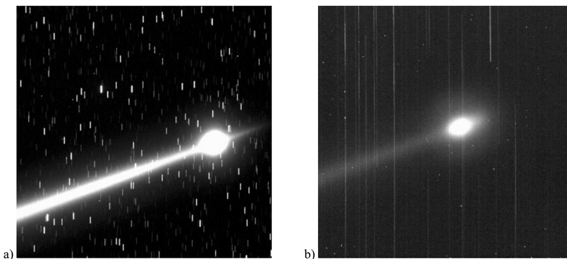
Figure 6: Images of the Teramobile laser beam (280 mJ, negatively chirped, unfocussed, 10 pulses/s) with a 2-m Schmidt telescope and a 4-Mpixel CCD. a) Pulse duration: 150 fs, filter: Johnson R, exposure time: 5 s, altitude range: 2.8 – 25 km. b) Pulse duration: 600 fs, filter: Johnson B + 2 mm BG 39, exposure time: 360 s, alt. Range: 2.9 – 42 km.
