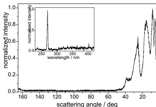
Figure 8: Angular distribution of the THG intensity generated in a water droplet (55  $\mu\text{m}$  diameter) excited with a pump wavelength of 810 nm. Inset: THG spectrum measured under  $30^\circ$ .
