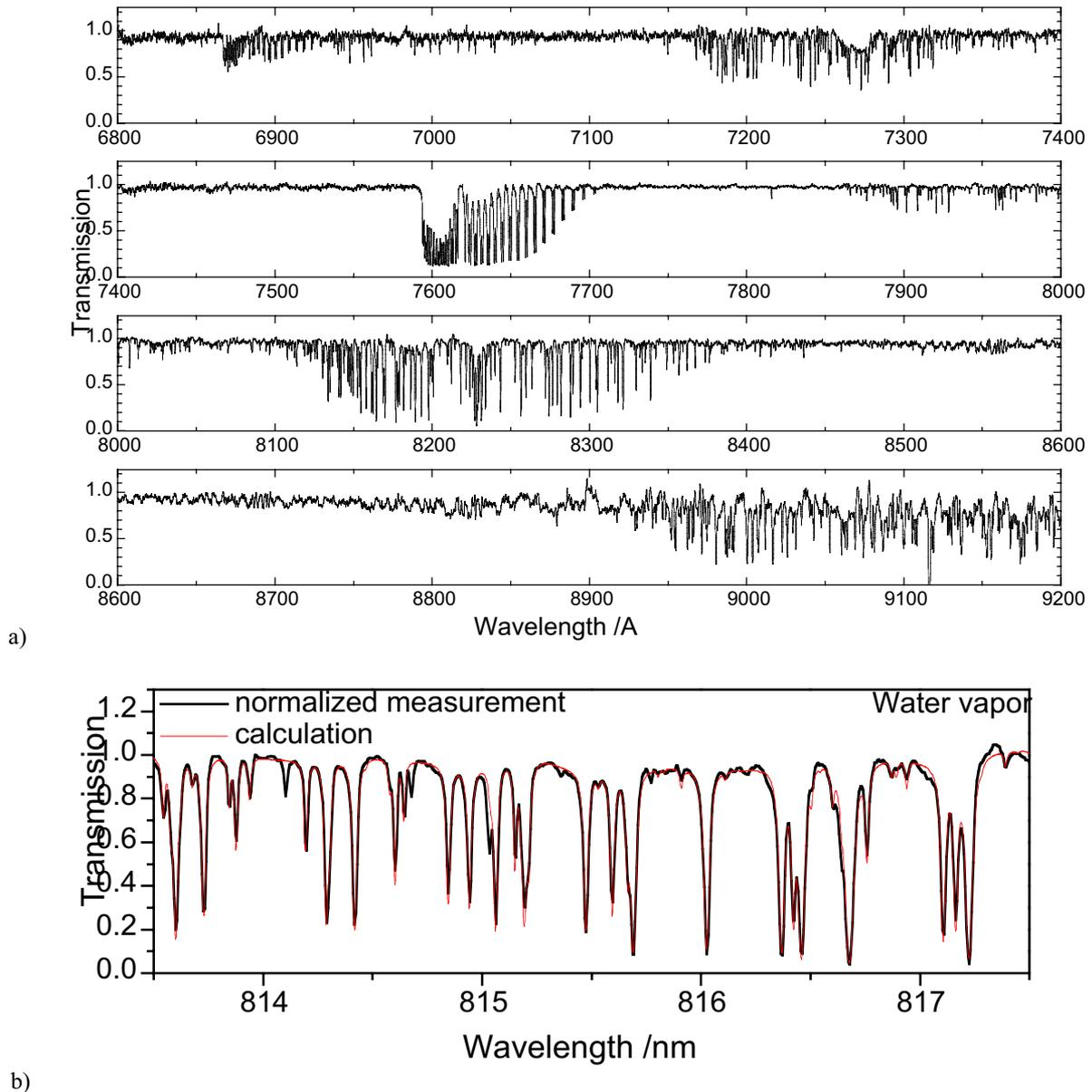
Figure 7: a) Absorption spectrum from one single exposure (backscatter altitude 4.5 km). b) Comparison of normalized measurement and calculation (after HITRAN) for a part of the  $\text{H}_2\text{O} (211)\leftarrow(000)$  vibration band.
