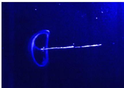
Figure 10: Haze formation in a diffusion cloud chamber along a plasma filament generated with a 1.5-mJ 60-fs laser (the laser pulses propagate from left to right).
