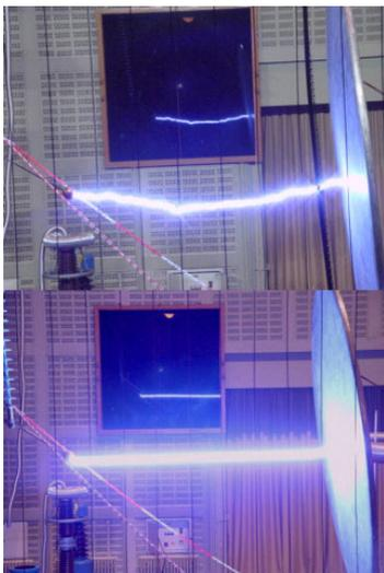
Figure 11: MV discharges between a neg. charged sphere and a grounded plane.
