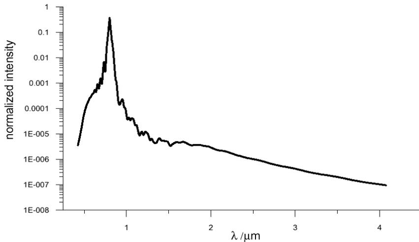
Figure 5: Simulated spectrum of an 85-fs pulse (10 mJ, 800 nm) after free propagation over 1.4 m in air. The radial symmetric calculation starts with a beam diameter of 0.7 mm.<sup>12</sup>
