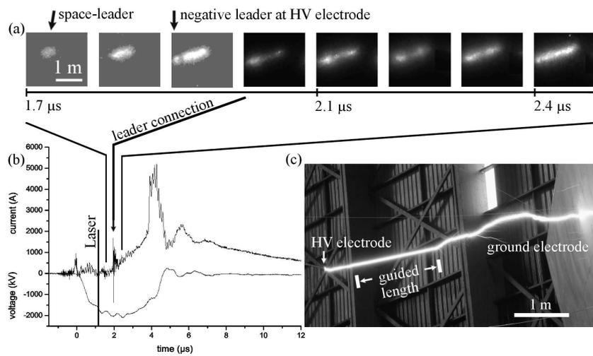
**Fig. 1** (a) a sequence of fast-frame camera pictures zoomed into the first part of the gap to show space-leader formation, (b) the corresponding records of the high voltage and current and (c) a still photograph of a partially guided discharge in a 4.5 m gap. The exposure time of each fast-frame picture was 40 ns with a delay of 50 ns between each.
