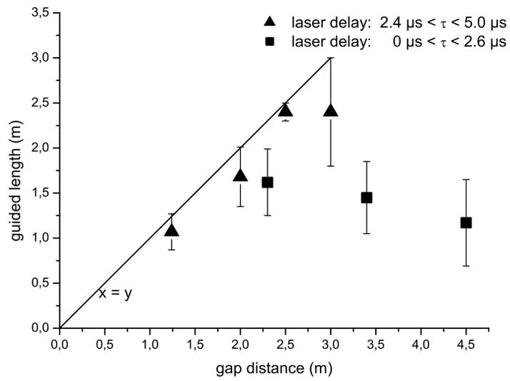
**Fig. 5** The mean values of the total guided lengths as a function of the gap distance.  $\tau$  denotes the time delay between the laser and the beginning of the voltage pulse, and the error bars indicate the standard deviation. The results for laser delays between 2.4 and 5.0  $\mu\text{s}$  were obtained in an earlier experiment [6].
