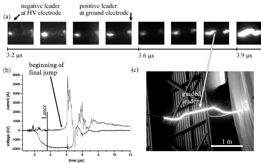
**Fig. 3** (a) a sequence of fast-frame camera pictures for a guided electrode leader in a 2.3 m gap, (b) oscillograms of a discharge with a guided electrode leader under similar conditions for a laser delay of 1.7  $\mu\text{s}$  and (c) a still photograph of the discharge.
