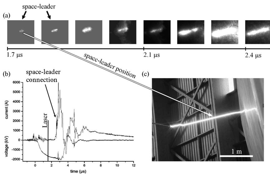
**Fig. 2** (a) a sequence of fast-frame camera pictures for a triggered space-leader in a 2.3 m gap, (b) oscillograms of a space-leader discharge under similar conditions for a laser delay of  $1.7 \mu\text{s}$  and (c) a still photograph of the discharge.
