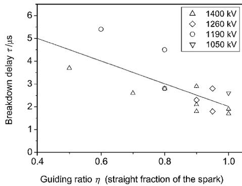
Fig. 3. Breakdown delay  $\tau$  as a function of the guided fraction of spark  $\eta$  measured with an electrode gap of 2 m. The linear fit yields a velocity  $v_g = (1.0 \pm 0.2) \times 10^6$  m/s for the guided propagation and a velocity  $v_f = (2.9 \pm 0.5) \times 10^5$  m/s for free streamer propagation.
