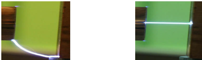
Left: spontaneous discharge in air between two electrodes with 30 kV/cm applied voltage. Right: discharge triggered by a self-guided femtosecond IR laser pulse. Applied voltage is 15 kV/cm. The distance between the electrodes is 2 cm.
