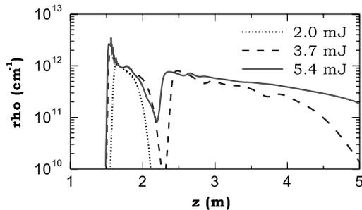
Fig. 7. Numerical simulations of the number of electrons per length unit ( $\rho$ ) for three different incident energies: 2, 3.7 and 5.4 mJ. The pressure is 0.6 atm. A super-Gaussian beam profile,  $I(r) \propto \exp[-2(\frac{r}{w_0})^n]$ , with  $n = 22$  and  $w_0 = 2.32$  mm, is used.
