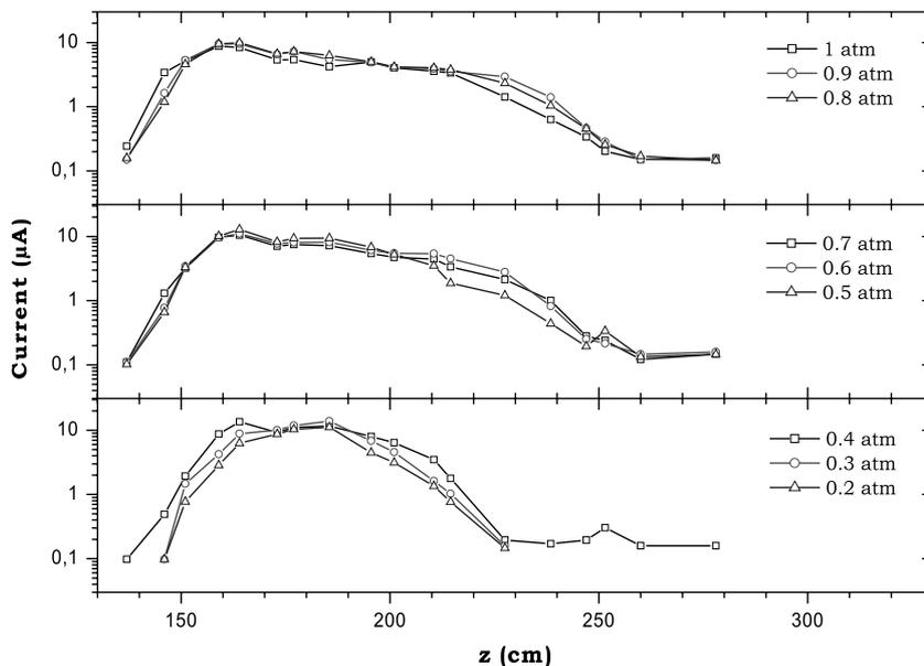
Fig. 5. Evolution of the conductivity of the filament along the optical axis with an energy equal to 3.7 mJ/pulse.  $z$  is the distance from the focusing lens. The presented signal corresponds to the current in the load resistance. The measurements have been performed for different pressures inside the tube, varying from 0.2 to 1 atm.
