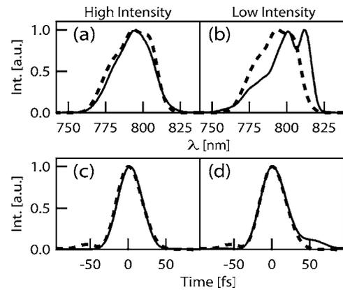
FIG. 2. Solid lines: experimental  $I(\lambda)$  and  $I(t)$  retrieved inverting the multi shot FROG measurement of [(a) and (c)] high and [(b) and (d)] weak intensity spots on the wavefront. Dotted lines: corresponding traces for a pulse propagating without turbulence over the same distance.
