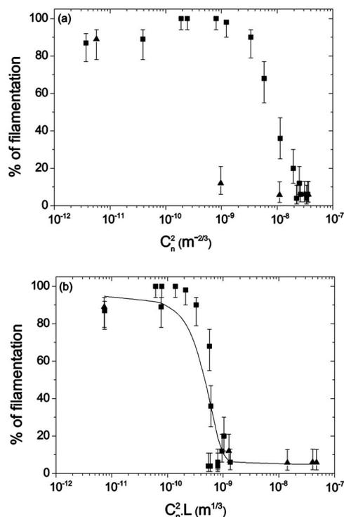
FIG. 1. Percentage of filaments surviving the turbulence as a function of  $C_n^2$ , in the case of localized (squares) and extended turbulent regions (triangles) located after the filament onset. (b) Same data plotted as a function of  $C_n^2 L$ ,  $L$  being the turbulence length. The line is intended to guide the eye.
