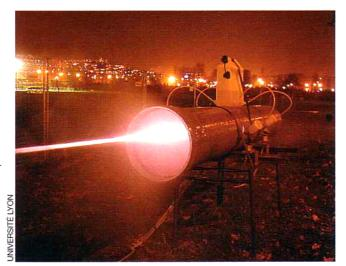
An ultrafast laser creates light filaments in the open air that propagate much as solitons propagate in fiber; in both cases, conflicting nonlinear processes create a pulse that neither diverges nor collapses.
