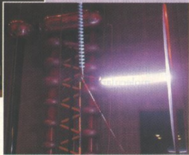
FILAMENT OF FIRE: The Teramobile laser [left] shoots pulses from a shed to the space between an electrode charged by a generating tower and a grounded electrode [not shown]. The pulse ionizes the air, creating a conductive filament. Artificial lightning follows the filament's straight path [below].
